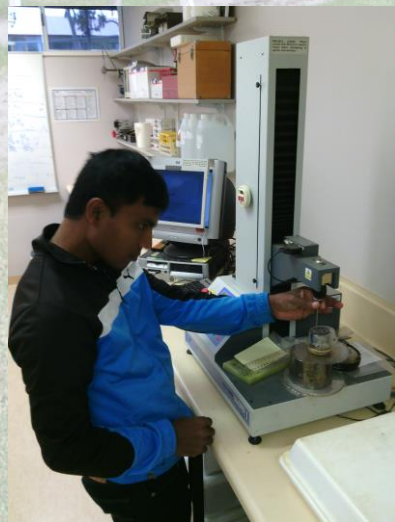
Gaus Azam determining soil penetration resistance of one of the samples.
